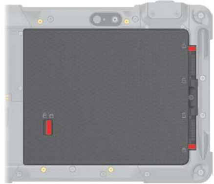
Incorrect (revealing red part)
